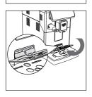
Lift the espresso tray off the grill of the drip tray and place it into the dedicated slot as shown in the drawing.
